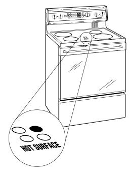
A "HOT SURFACE" light will glow brightly when any element is turned on.
